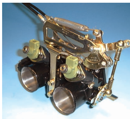
Alpha throttle body top mounting linkage
